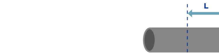
A marking for visual control of the push-in length is optional. The Push-In length is mentioned in Table 3. In cases the tube is not pushed in correctly, and only passing the grip ring (see above), a measurable controlled leakage will occur. An audible whistle can be heard to locate. Depending on the dimension the tube can be repushed under pressure, to secure a 100% assembly.
